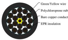
Polychloroprene rubber outer jacket Bare copper conductor
